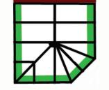
Denotes the area covered by the insulated pelmet (orangery sections). Please note that the Orangery section widths will vary dependant on roof pitch.
