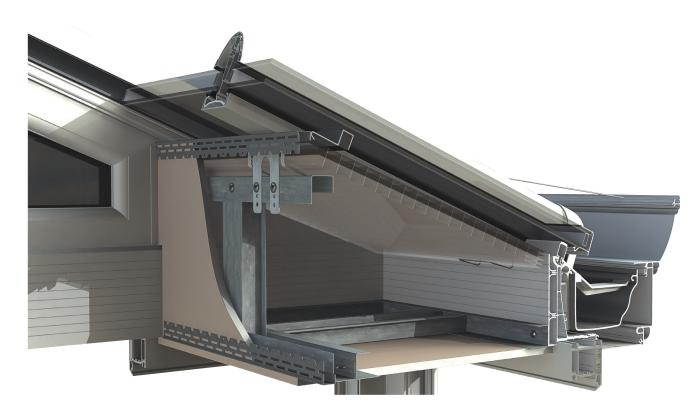
If this is a new installation of an insulated internal pelmet then the design of the gable frame should cover the 'open end' of the ladder framework. On retro fits where a redesign of the gable feature is not feasible, the application of a privacy film to the glass may suffice.
